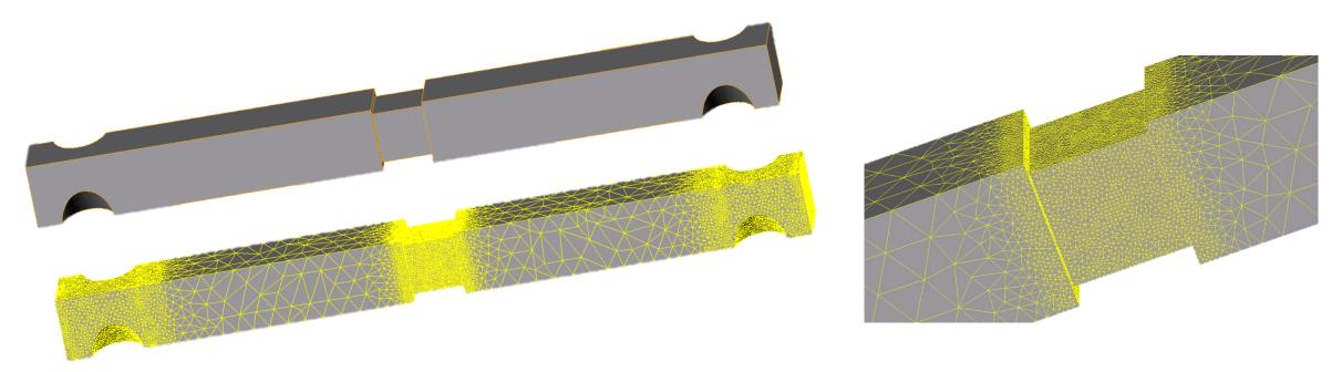
Simulation of a model made of simple elements (triangles, squares, tetrahedrons, cubes) significantly smaller than the size of the original body
